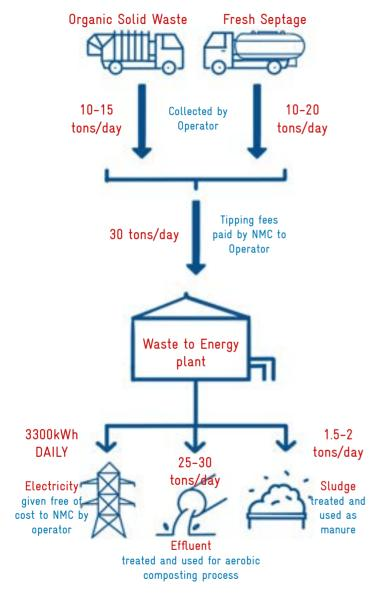
Schematic of the Waste to Energy Process
